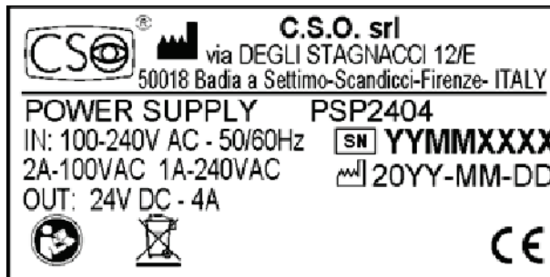
Fig 3 - Power supply PSP2404 data plate
